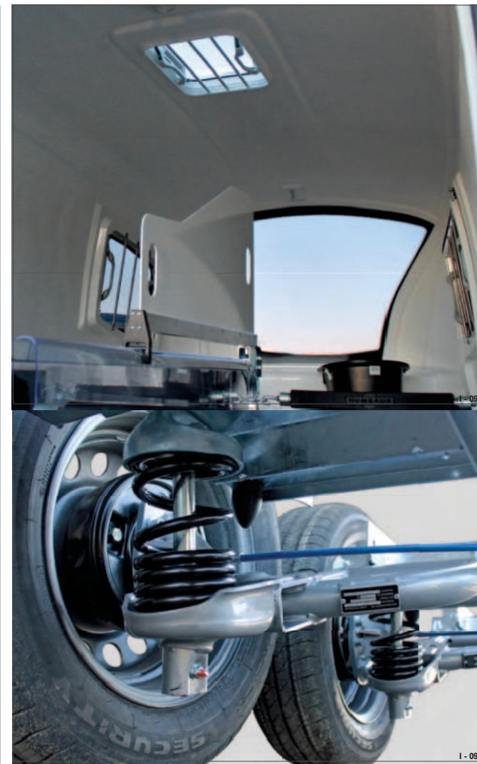
Fig. 21 EquiDrive PLUS S - spiralfjädring
