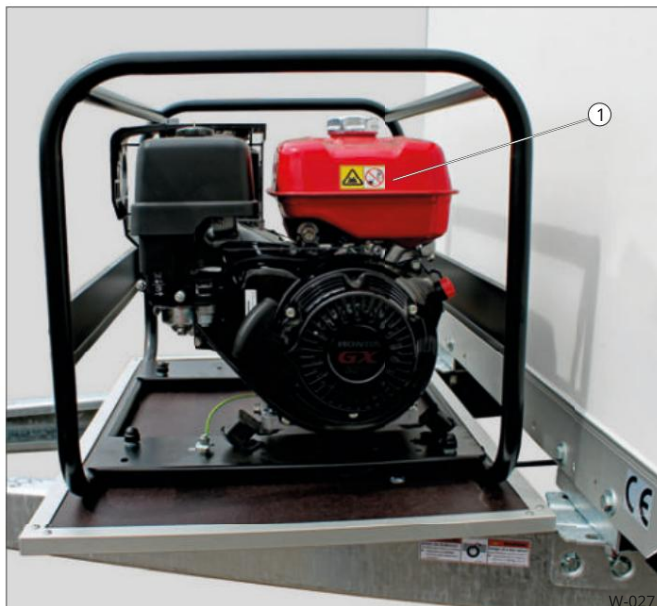
Sl. 28 Generator snage 1 spremnik goriva
