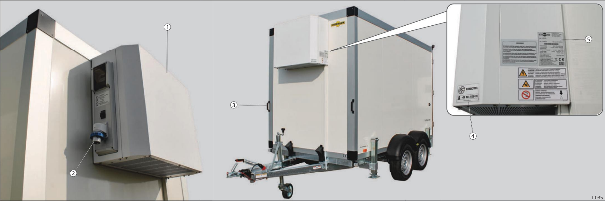
Sl. 37 Tandem rashladni sanduk s Humbaur jedinicom
