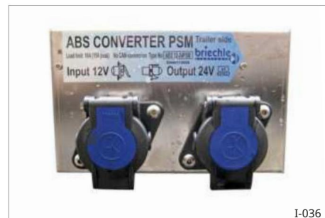
Sl. 29 Naponski transformator EBS / ABV
