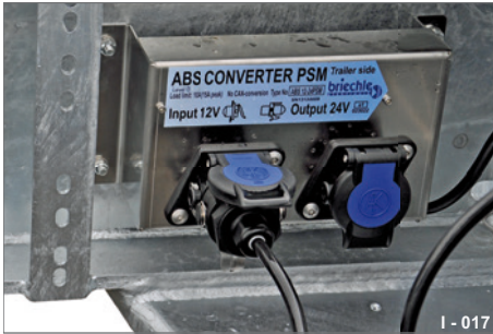
Abb. 17 ABS Converter 24 V / 12 V
